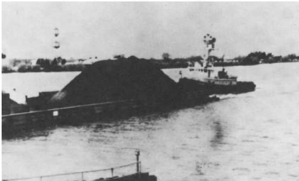
Figure 3-2. Tugboat and barge transporting dredged material
